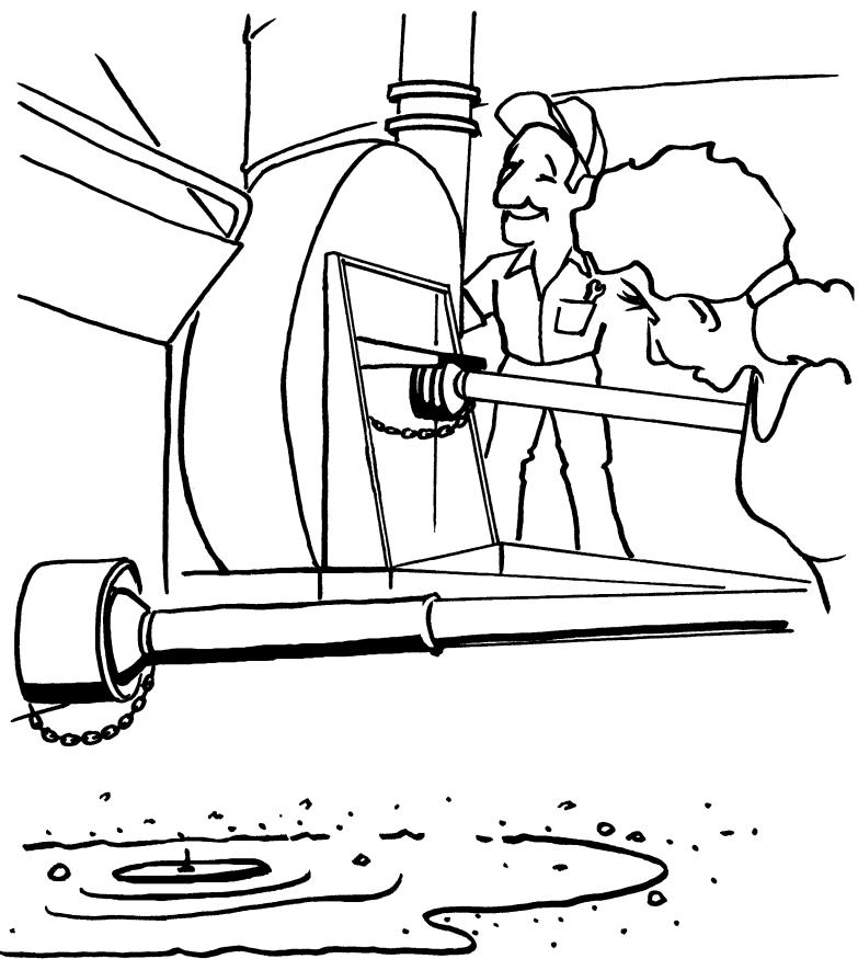
It's a little muddy here. Before someone slips and falls into the driveline or the machines, I'll put sawdust or straw down to improve the footing. Finding time for safety makes good sense.
