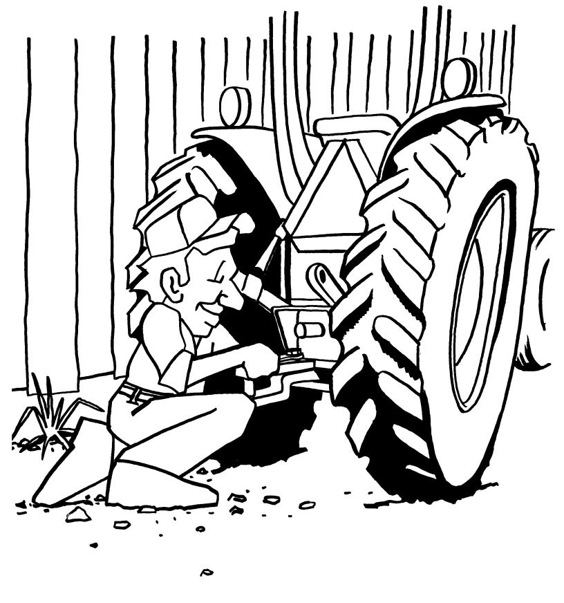
Strap hitches are good for tillage work but must be removed to avoid damage to PTO driveline guards.
