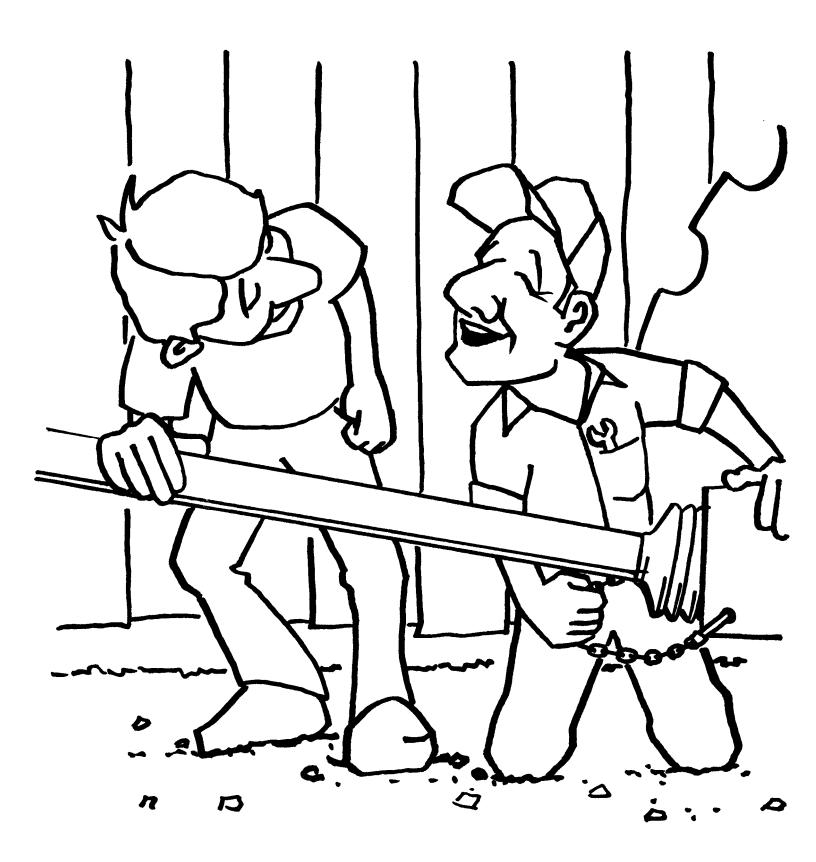
This chain is provided to keep the guard from rotating during operation. Attach it with enough slack to allow for tight cornering.
